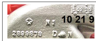
All cast engine parts will have some type of date code on them. Depending on the casting plant, how worn the mold is or how worn the part itself is it may be challenging to read the date
