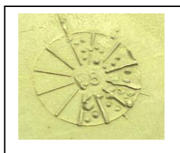
1969 alternator #28757749. The assy date is 34 th week of 1968 (Aug 17-21). casting date= 7 th month of 1968. Difference of 30 days (casting to assy)
