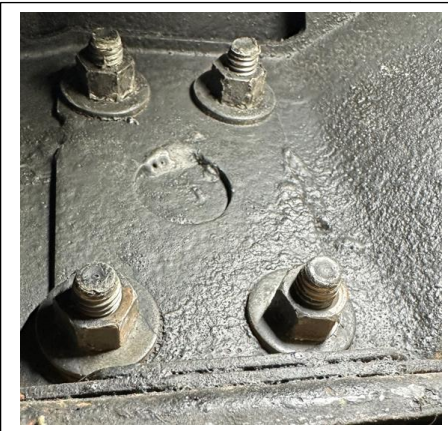
Factory original frame reinforcements at leaf springs with torque boxes and plates, front frame to rocker supports. Rh rear frame rail die lot stamp number is RT 38-1 & TSL38-1
