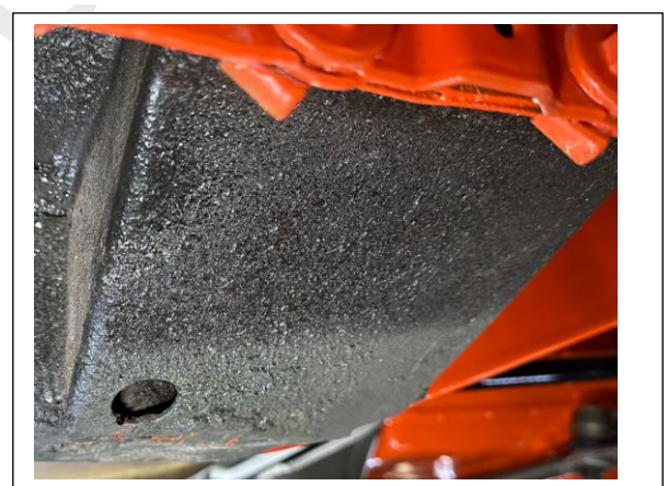
Factory original torque boxes with inner and outer plates.
