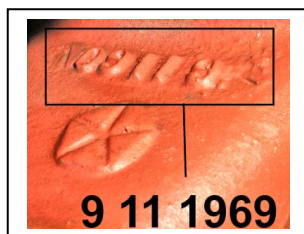
All cast engine parts will have some type of date code on them. Depending on the casting plant, how worn the mold is or how worn the part itself is it may be challenging to read the date
